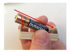
3. Slide the battery tray back into the flashlight body with the positive side facing the LEDs side. You will find the '+' sign on the battery tray stamped on the metal edge. Incorrect installation of battery tray may cause damages to the lamp!
